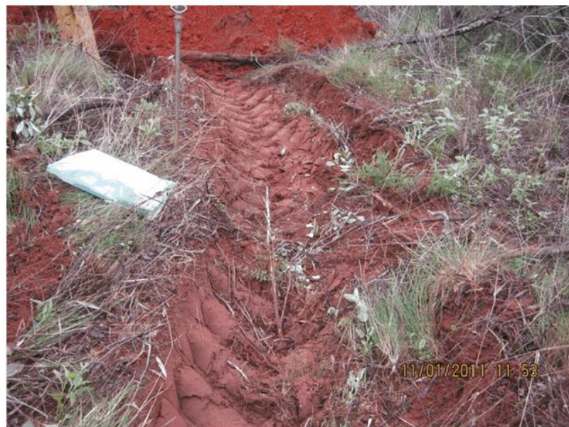
Photograph 2: Very loose soil evident from backhoe tracks (TP06)
