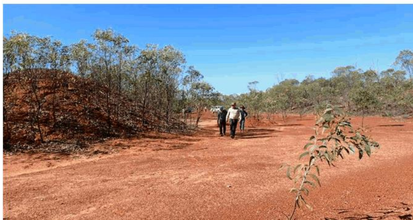
Photo 4 - Typical Conditions at the Lateritic Gravel Pits. Excavated pindan sand overburden is stockpiled (left side of the photo) Lateritic gravel has been quarried (i.e. gravel not visible on the photo) Base of pit comprises the Melligo sandstone surface.
