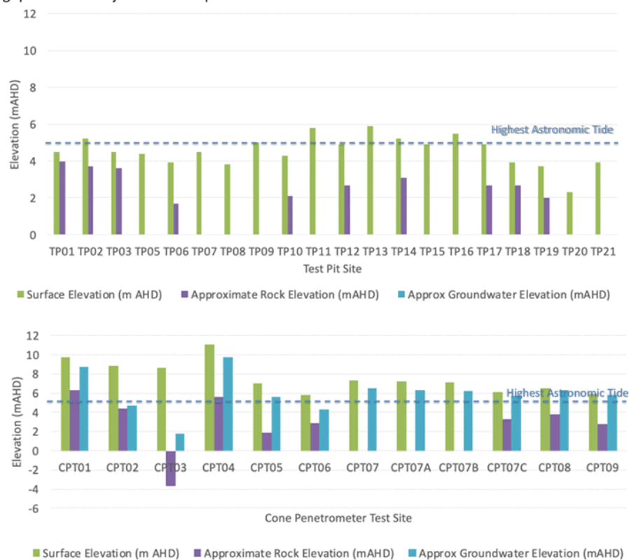
Figure 2.3 Compiled Surface, Rock and Groundwater Elevations (mAHD) from test pits above (above) and CPTs (below), interpreted from Galt 2020.
