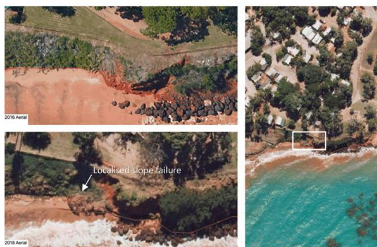
Figure 4.9 Pindan Headland showing localised slope failure between 2016 and 2018
