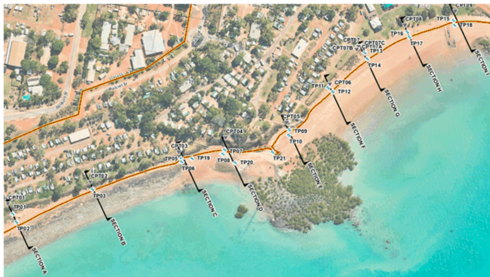
Figure 2.1 Geotechnical Sampling Sites including Test Pits (TP) and Cone Penetrometer Tests (CPT).
