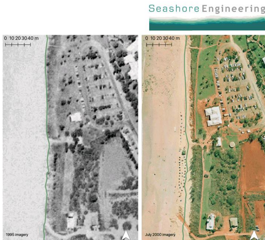
Figure 3.7 Comparison of aerial imagery from 1995 to July 2000. Assumes most of the change is associated with impact of TC Rosita, noting there is 5 years between dates of imagery.
