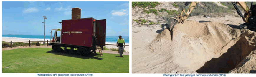
Figure 2.3 Cable Beach Geotechnical Investigation: Cone Penetrometer Tests along the Dune Crest (left) and Excavated Test Pits on Beach (right)
