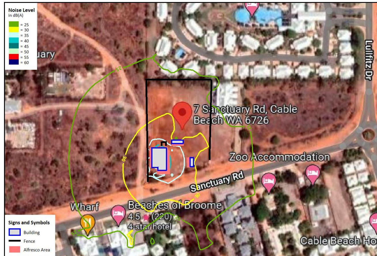
Figure 9: Worst-case noise level contours for scenario 4.
