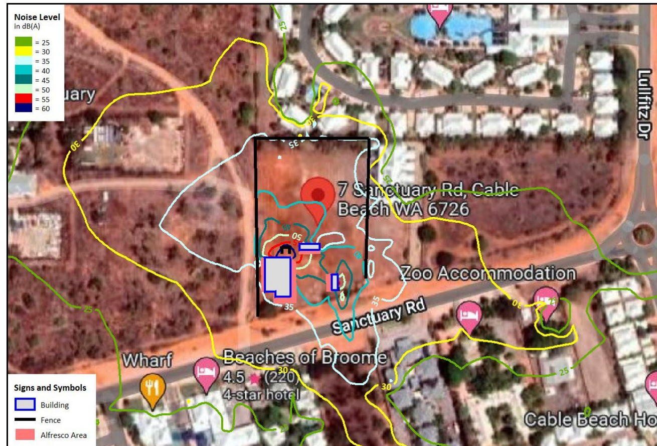
Figure 5: Worst-case noise level contours for scenario 1.
