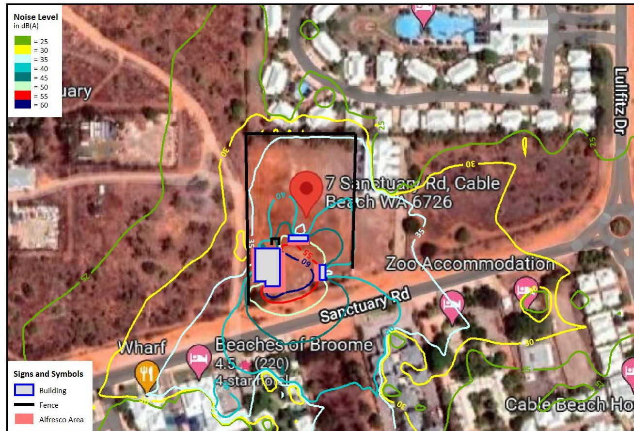
Figure 7: Worst-case noise level contours for scenario 3.
