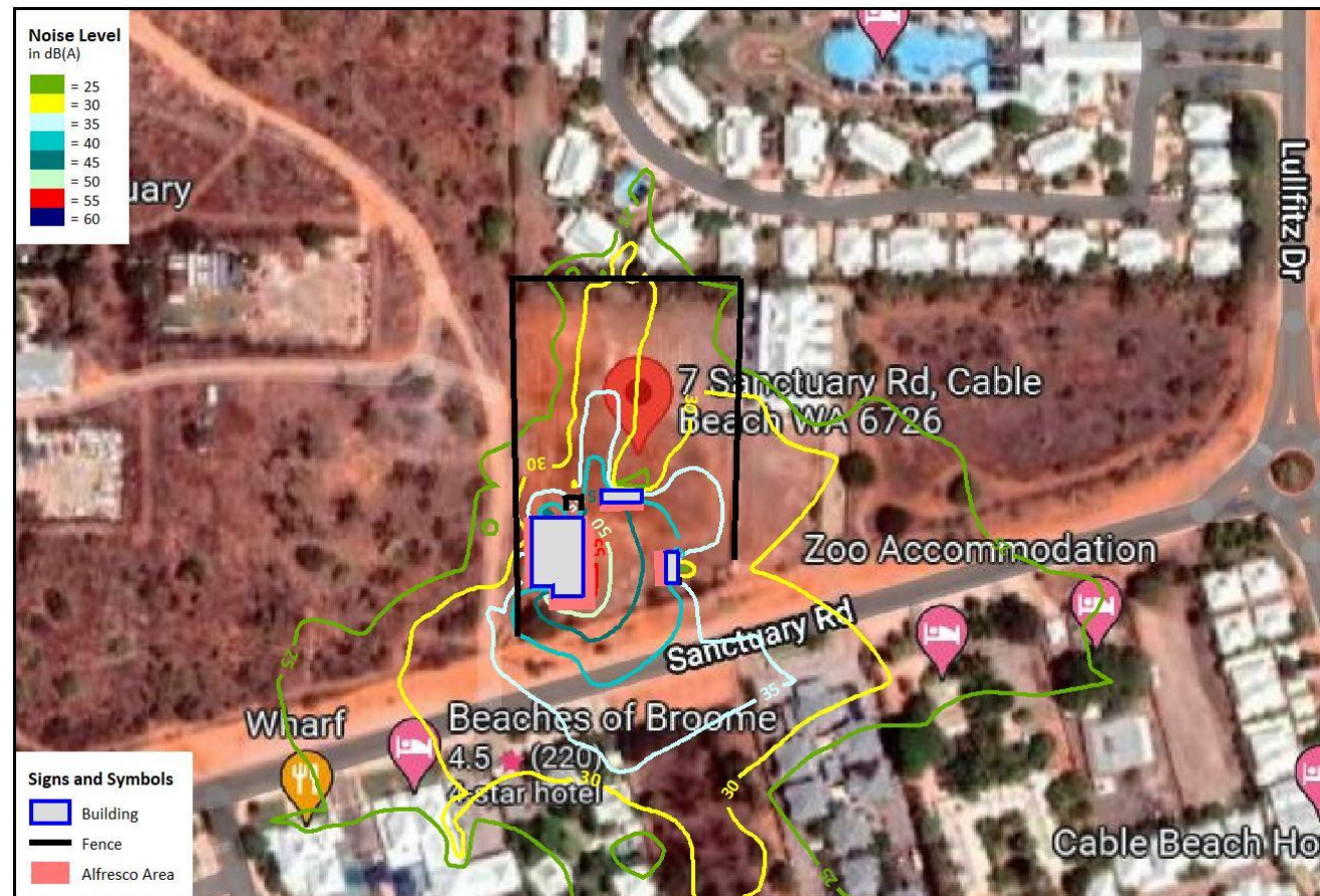
Figure 6: Worst-case noise level contours for scenario 2.
