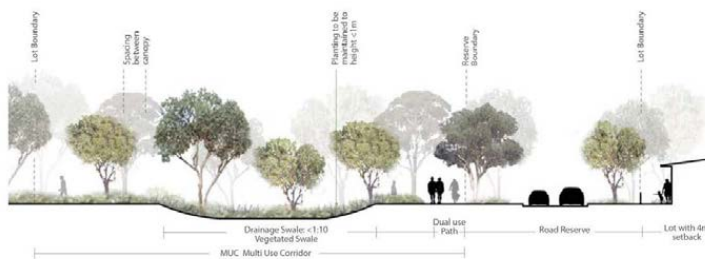
Indicative cross-section for MUC Source: Local Development Plan 3 Broome North
