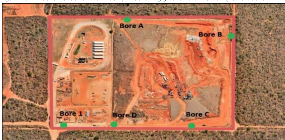
Figure 10.1 Extract of Schedule 1 from Facility EPL, showing groundwater monitoring bore locations
